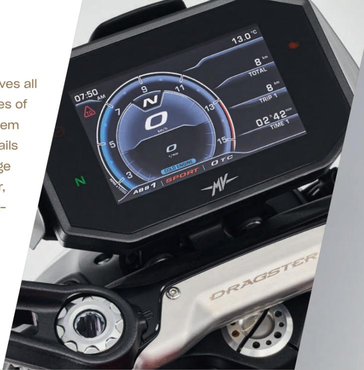
The MVICS with full Ride-By-Wire has been further improved. The rider can make use of eight levels of traction control, and four riding modes, namely Sport, Race, Rain, and Custom, the last of which can be significantly customised to suit the riding style and tastes of the individual. Changing the character of the engine has never been so quick and intuitive, like having four bikes in one.
