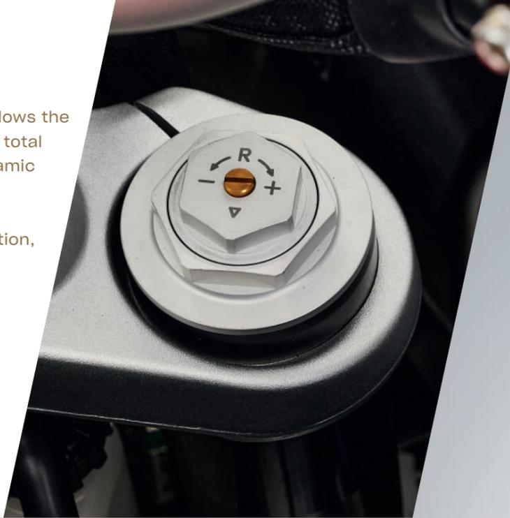
The Turismo Veloce project prioritises riding pleasure and the ability to adapt to different styles and conditions of use. Hence, the Rosso version also allows for significant suspension adjustment. In particular, the Marzocchi fork with 43 mm stanchions can be adjusted separately in its compression and rebound damping, as well as its spring pre-load. And the Sachs shock absorber connected to the elegant swingarm in aluminium alloy offers the same adjustment.
